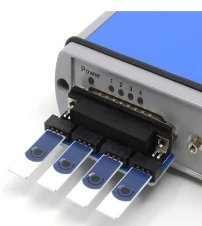
Figure 4. Cyclic voltammetry (CV) for label-free analysis of NM effects. CV voltage is swept from one value to another, and then back again, resulting in a current as a function of voltage and scan rate. It provides information about electrochemical reactions (redox) occurring at the working electrode. CV can be used to monitor oxidation and metabolism of ascorbic acid (AA).
